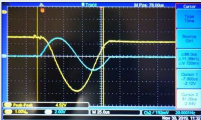
Figure 10: PK Vesp and I pulse waveform. Vesp 14kV/1V , Ipulse 100A/1V
